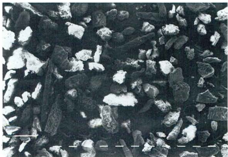
Fig. 2. - Talc i altres partícules presents a la mostra. Marques: 10 \mu\text{m} (x 400). Fig. 2. - Talc and other particles present in the sample. Markers: 10 \mu\text{m} (x 400).
