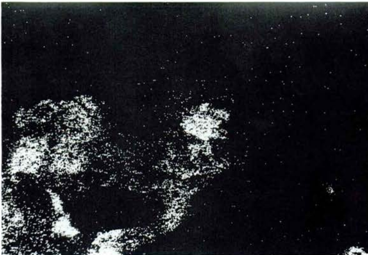
Fig. 32. - Mapping de Ca corresponent a la mateixa zona de la figura anterior. Fig. 32. - Ca mapping corresponding to the same zone as in the above figure.
